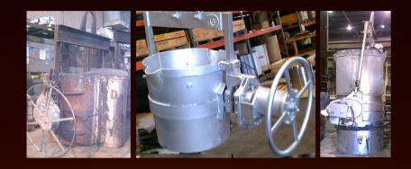
Del Sol proudly represents D&E Foundry Ladles. D&E is known for making high quality, robust ladles. D&E uses Dodge gearboxes as standard featuring an automatic locking mechanism to keep the ladle from freewheeling.
